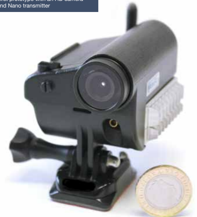
First prototype with an HD camera and Nano transmitter
